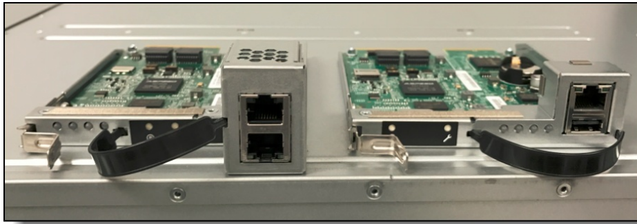
Figure 15. Dual-port SMM and standard (single-port) SMM
